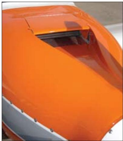
Two views of the intercooler's top cowl flap: closed on the ground (left) and open during climb. The drag of the necessary flap is measurable.
