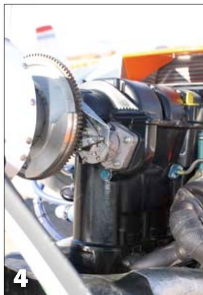
4. The inverted design places the crankshaft line properly for aircraft intended to use flat-opposed engines. Notice the standard prop governor and balance weight integrated into the starter ring gear.
