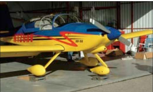
To be sure about weights, the Van's factory RV-9A is placed on electronic scales; the Wilksch was weighed immediately after. The diesel aircraft is actually 57 pounds lighter overall.
