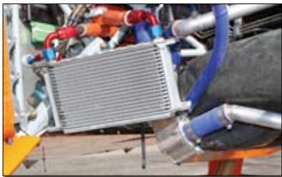
The oil cooler is fed air from a side-mounted NACA duct.
