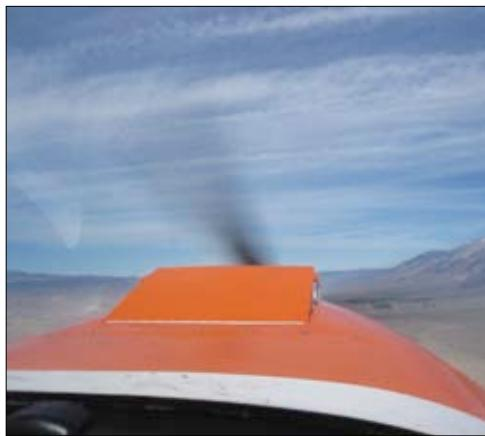
The additional drag of the open cowl flap is measurable and would explain why the climb rate of the WAM RV-9 was not as good as might otherwise be expected. (For perspective, consider that the climb rate of many "high-performance" certificated aircraft is comparable to that of the WAM RV-9. It's just that the "big engine" Lycoming RV-9A with the constant-speed prop has climb performance most people only dream about.)
