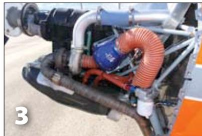
2. The air-to-air intercooler is visible through the duct. Reducing inlet-air temperature is key to obtaining good power and reliability.
